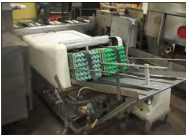
Figure 13. Automatic plastic egg flat washer washes, rinses, and stacks egg flats for drying after each use. (00CN0051)
