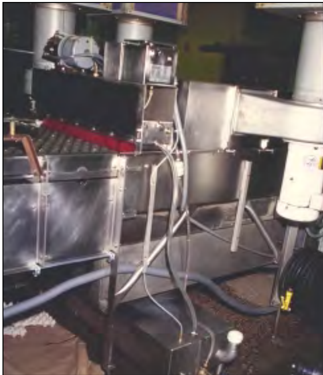
Figure 12. Food-grade mineral oil is pumped from reservoir (floor tank) to high-pressure spray nozzles to provide a light coating over each egg. (00CN0050)
