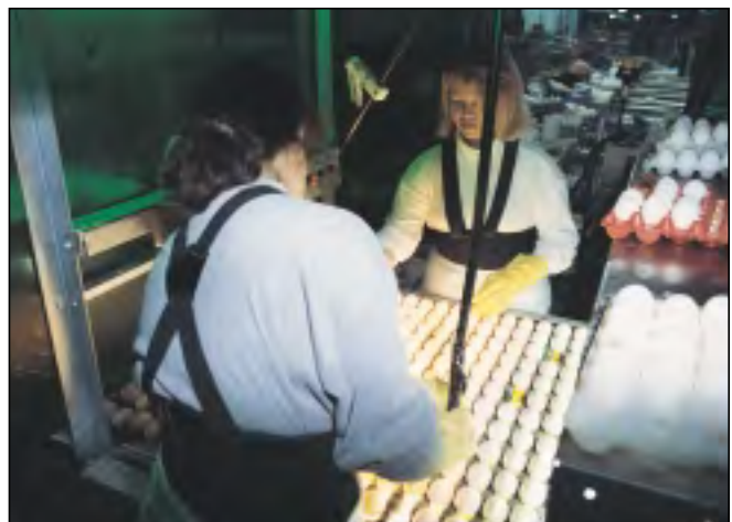
Figure 15. During candling, a wand-type pointer electronically marks eggs that are dirty or cracked, or that contain blood spots. Newer equipment is capable of automatically removing these eggs with minimal oversight. (99-CD-1606)
