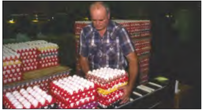
Figure 5. Flats of eggs are loaded onto the washing line at the off-line conveyor. (CD 8202 3241 1143-25)
