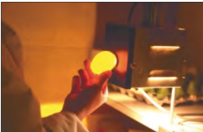
Figure 50. USDA grader demonstrating the use of a hand candling light. (CD 8202 3241 1143-14)
