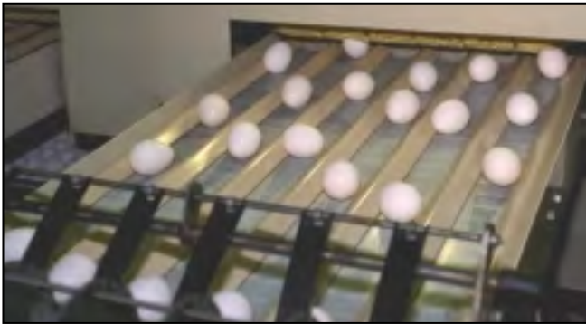
Figure 17. Eggs are automatically conveyed to packaging unit. (CD 8202 3241 1143-27)
