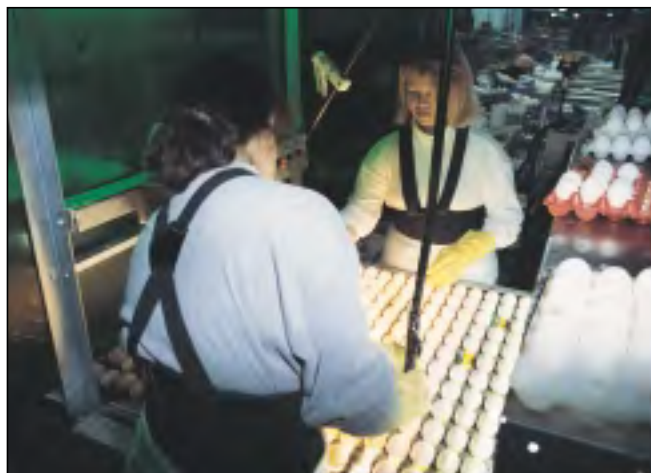
Figure 15. During candling, a wand-type pointer electronically marks eggs that are dirty or cracked, or that contain blood spots. Newer equipment is capable of automatically removing these eggs with minimal oversight. (99-CD-1606)
