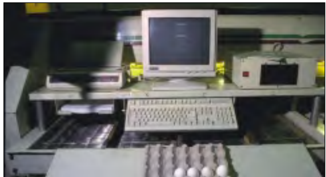
Figure 21. A computer attached to the processing system monitors and controls each phase of processing. (CD 8202 3241 1143-55)
