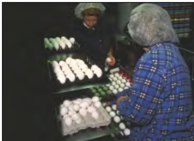
Figure 14. Plant personnel segregate broken and dirty eggs after the washing cycle and prior to the candling operation. (CD 8202 3241 1143-1)
